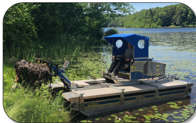
Image 4: An Aquatic weed managers uses an amphibious machine to remove dense beds of invasive waterlily.
